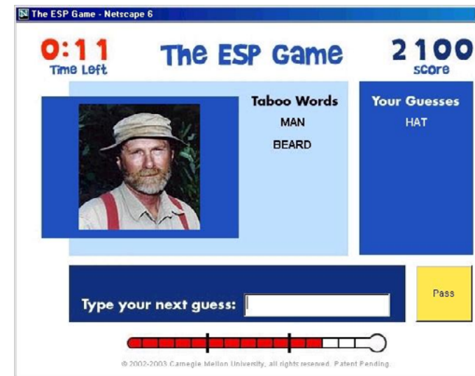
Fig. 4 The interface of the ESP Game. The thermometer at the bottom measures how many images partners have agreed on. When filled, players gain a bonus point.
