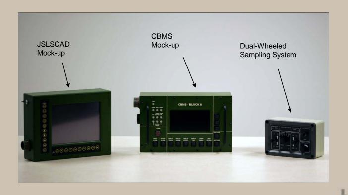
Hands-On Mockup Devices provide low-cost, realistic simulation of complex sensors. These simulated devices can be used for **stand-alone individual training**, and with the combined America's Army environment for **collective training**.
